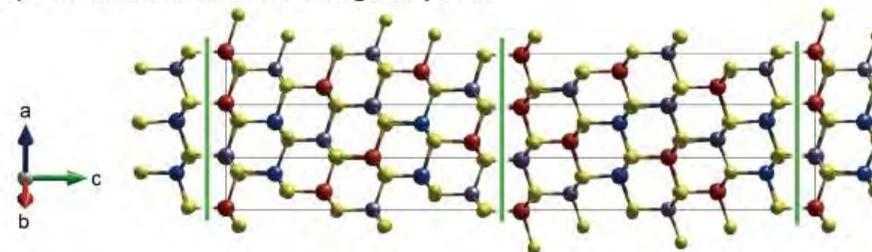
c) Coherent interfaces between the orthorhombic and tetragonal phases
