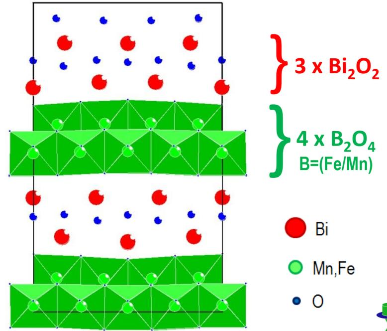
$Amm2$  (SG n°38)  $a=3.96\text{\AA}$ ,  $b=11.78\text{\AA}$  and  $c=19.37\text{\AA}$
