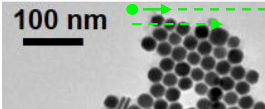
1- scan a tiny parallel beam on nanoparticles and collect ED.
