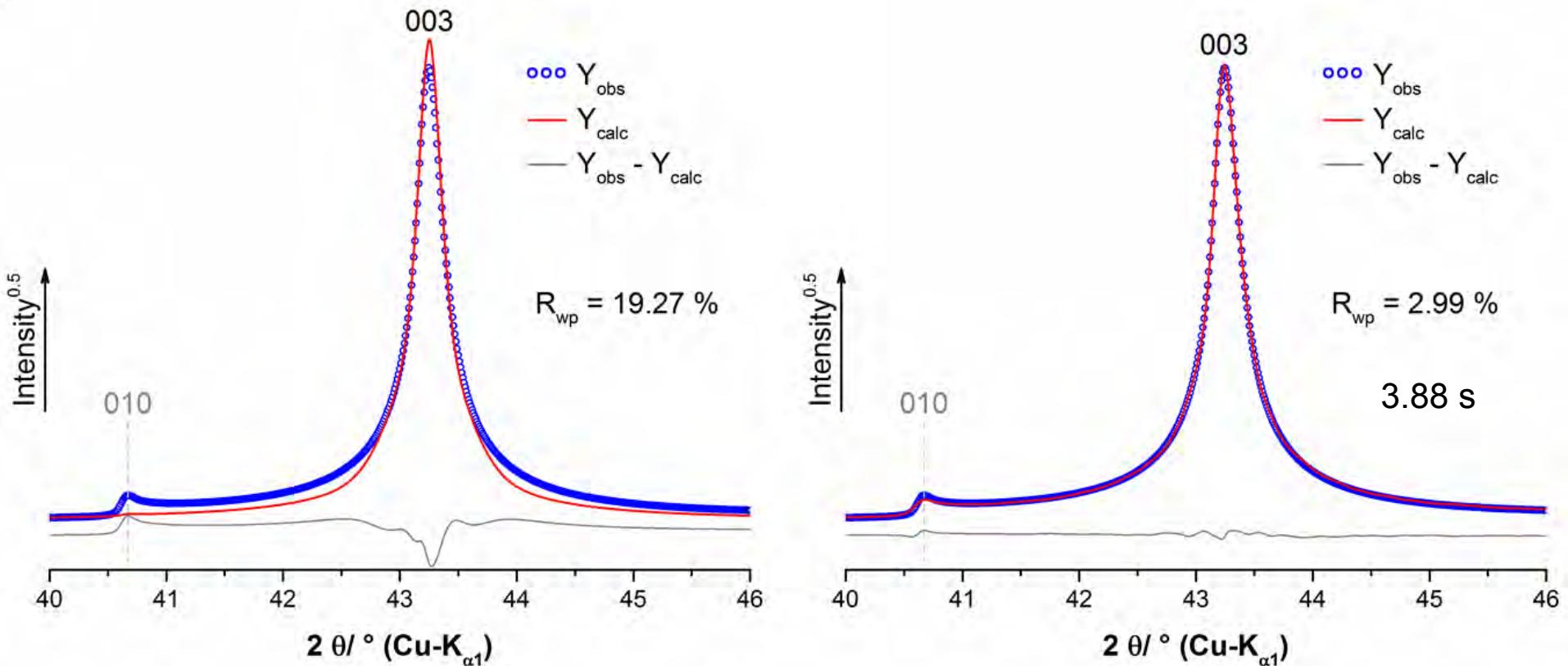
1 out of 100 Rietveld refinements using the faultless structure (left) and a 5000 layer supercell (2 % fault probability)
